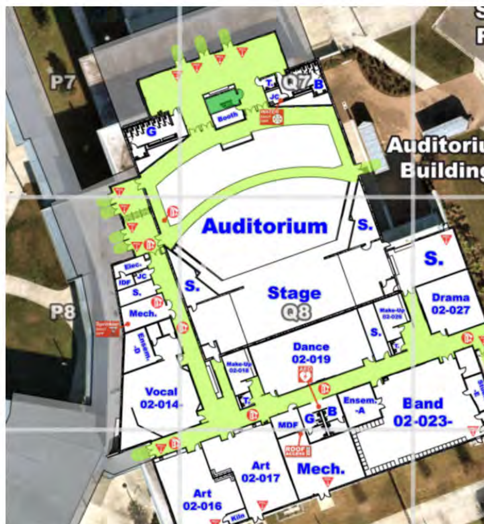
Asset locations for fire alarm pull stations, AEDs and fire extinguishers overlaid on a CRG
