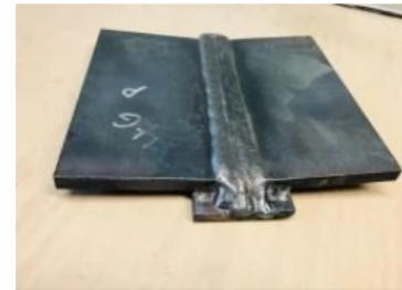
AWS D1.1 Structural Steel Student will demonstrate ability to weld carbon and low-alloy metals
