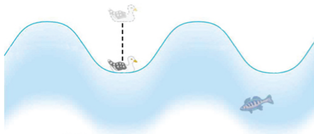
Figure 13.2 An idealized ocean wave passes under a seagull that bobs up and down in simple harmonic motion.
