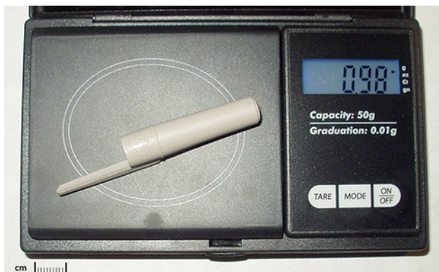
Figure 1.20 Whereas a mechanical balance may only read the mass of an object to the nearest tenth of a gram, some digital scales can measure the mass of an object up to the nearest thousandth of a gram. As in other measuring devices, the precision of a scale is limited to the last measured figures. This is the hundredths place in the scale pictured here. (credit: Splarka, Wikimedia Commons)
