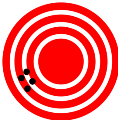
Figure 1.22 In this figure, the dots are concentrated close to one another, indicating high precision, but they are rather far away from the actual location of the restaurant, indicating low accuracy. (credit: Dark Evil)
