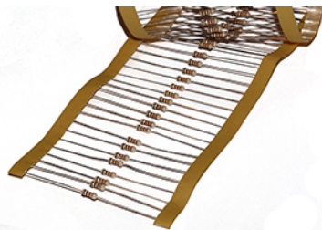
Figure 19.11 Some typical resistors. The color bands indicate the value of the resistance of each resistor.
