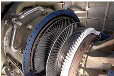
Figure 20.40 Steam turbine generator. The steam produced by burning coal impacts the turbine blades, turning the shaft which is connected to the generator. (credit: Nabonaco, Wikimedia Commons)
