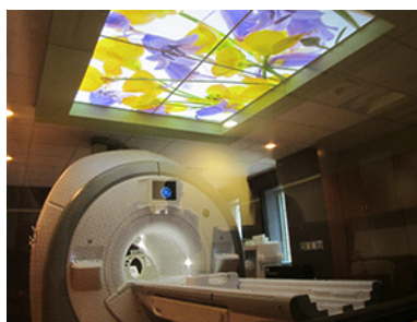
Figure 20.13 Instrument for magnetic resonance imaging (MRI). The device uses a cylindrical-coil electromagnet to produce for the main magnetic field. The patient goes into the “tunnel” on the gurney. (credit: Bill McChesney, Flickr)
