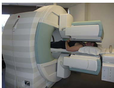
Figure 22.44 SPECT uses a rotating camera to form an image of the concentration of a radiopharmaceutical compound. (credit: Woldo, Wikimedia Commons)
