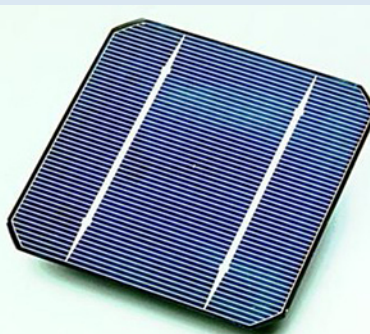
Figure 21.10 A solar cell is an example of a photovoltaic cell. As light strikes the cell, the cell absorbs the energy of the photons. If this energy exceeds the binding energy of the electrons, then electrons will be forced to move in the cell, thereby producing a current. This current may be used for a variety of purposes. (credit: U.S. Department of Energy)
