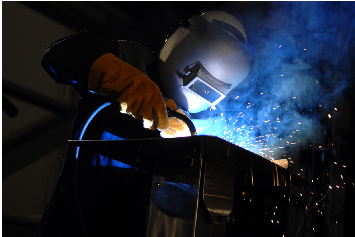
Figure 11.1 The welder's gloves and helmet protect the welder from the electric arc, which transfers enough thermal energy to melt the rod, spray sparks, and emit high-energy electromagnetic radiation that can burn the retina of an unprotected eye. The thermal energy can be felt on exposed skin a few meters away, and its light can be seen for kilometers (credit: Kevin S. O'Brien, U.S. Navy)
