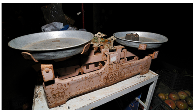
Figure 1.19 A double-pan mechanical balance is used to compare different masses. Usually an object with unknown mass is placed in one pan and objects of known mass are placed in the other pan. When the bar that connects the two pans is horizontal, then the masses in both pans are equal. The known masses are typically metal cylinders of standard mass such as 1 gram, 10 grams, and 100 grams. (credit: Serge Melki)
