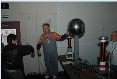
Figure 18.13 The man touching the Van de Graaff generator has excess charge, which spreads over his hair and repels hair strands from their neighbors. (credit: Jon ‘ShakataGaNai’ Davis)
