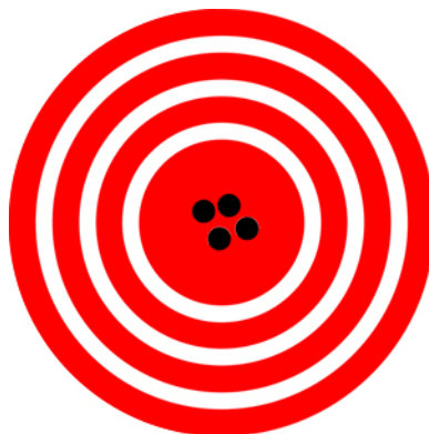
Figure 1.23 In this figure, the dots are concentrated close to one another, indicating high precision, but they are rather far away from the actual location of the restaurant, indicating low accuracy. (credit: Dark Evil)
