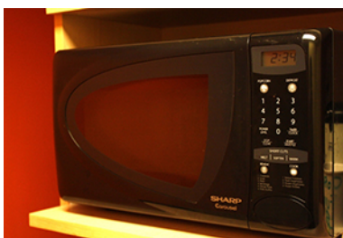
Figure 1.7 Microwave ovens use electromagnetic waves to heat food. (credit: MoneyBlogNewz)
