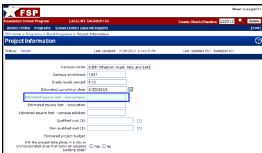
Slide 89 If the project will construct a completely new campus, enter the campus's square footage in the *Estimated square feet - new campus* field.
