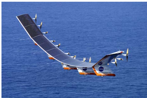
Figure 7.22 Solar energy is converted into electrical energy by solar cells, which is used to run a motor in this solar-power aircraft. (credit: NASA)
