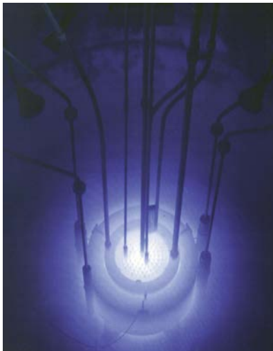
Figure 17.21 The blue glow in this research reactor pool is Cerenkov radiation caused by subatomic particles traveling faster than the speed of light in water. (credit: U.S. Nuclear Regulatory Commission)
