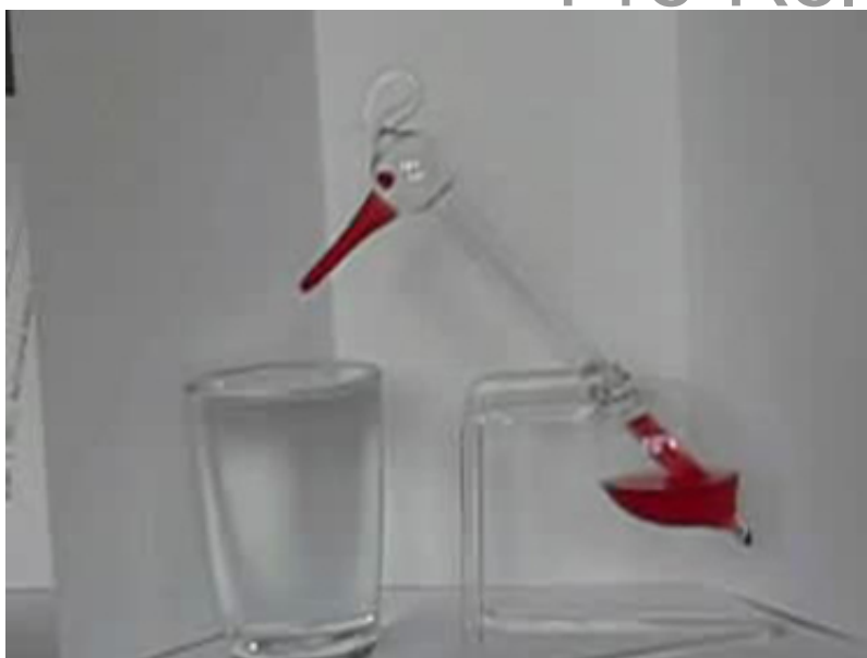
Figure 15.22 This novelty toy, known as the drinking bird, is an example of Carnot's engine. It contains methylene chloride (mixed with a dye) in the abdomen, which boils at a very low temperature—about 100^{\circ}\text{F} . To operate, one gets the bird's head wet. As the water evaporates, fluid moves up into the head, causing the bird to become top-heavy and dip forward back into the water. This cools down the methylene chloride in the head, and it moves back into the abdomen, causing the bird to become bottom heavy and tip up. Except for a very small input of energy—the original head-wetting—the bird becomes a perpetual motion machine of sorts. (credit: Arabesk.nl, Wikimedia Commons)
